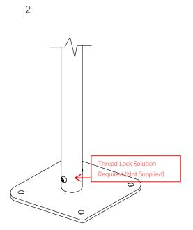
Fix instrument to Surface fix plate using M10 bolt and Barrel Nut and use **thread locking solution** to prevent fixings working loose.
